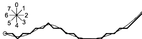
Figure 6.3 Freeman chain coding. Only the first coordinate pair is stored (x,y) together with a sequence of directions each coded by a single integer as shown.
